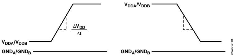
Figure 13. Transient Immunity Waveforms—Output Supplies
